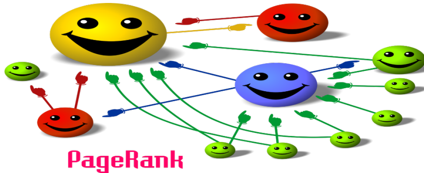
Figure 4: The size of each face is proportional to the total size of the other faces which are pointing to it.
